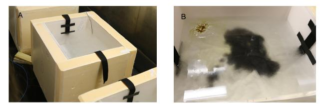
Figure 2. Ice tank mesocosms A. Clean ice tank; B. Oil encapsulated in the ice
