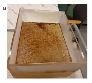
Figure 4. Ice mesocosm of water accommodated fraction and dispersant (WAF+CE). A. Bottom tap bottle with WAF+CE; B. Ice formation from WAF+CE.
